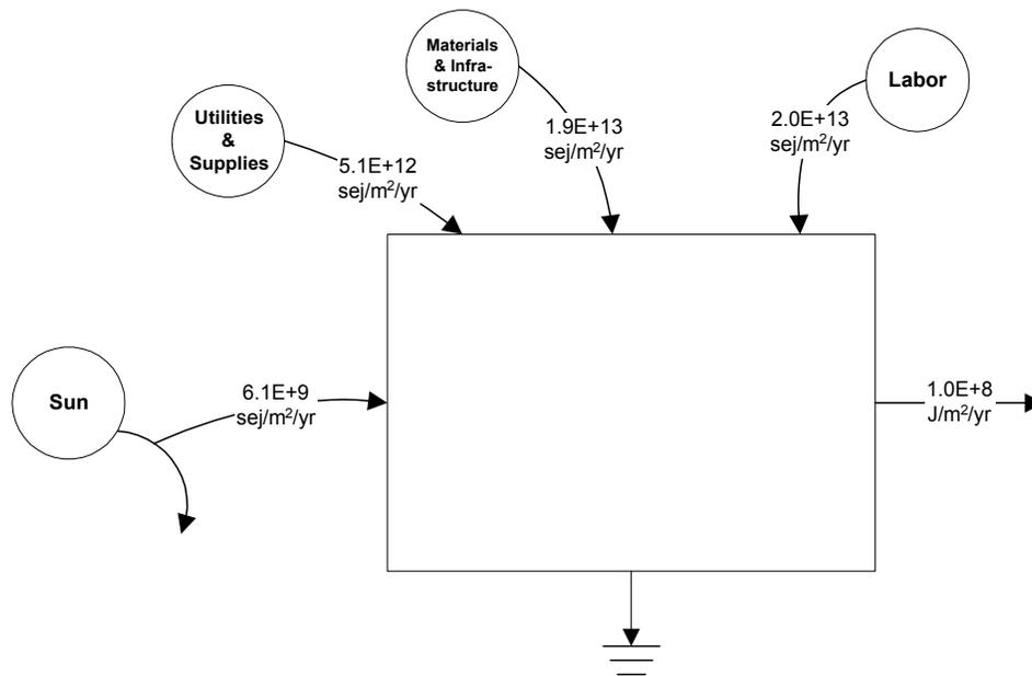
**Figure 1.** Emergy budget developed to reanalyze H.T. Odum’s original analysis of a pilot-scale algae plant for food production.
