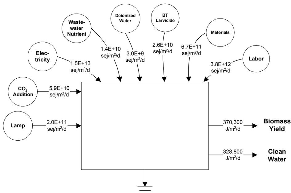
**Figure 4.** Energy budget diagram of the USDA algal turf scrubber, used to calculate the transformity of the outputs.
