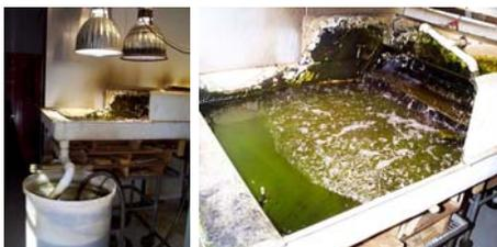
Figure 1: Laboratory-scale algal turf scrubber. Recycled effluent is continuously pumped into a wave surge bucket from a plastic drum below. The bucket fills and tips every 15 s. The effluent washes over the turf screen before draining into the drum below to be recycled. Water depth over the screen is 1–2 cm. Metal halide lamps are located approximately 42 cm above the growing turf.
