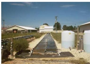
Figure 2: Pilot-scale ATS raceways at the Beltsville Dairy Research Unit.
