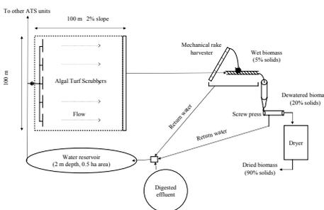
Figure 4: Schematic diagram of 1 ha ATS unit with associated equipment and water reservoir. Manure effluent is added continuously to equalization reservoir. Algal biomass is harvested weekly, removed from ATS effluent using a mechanical rake, dewatered with a screw press, and dried using a drum drier. A 1000-animal farm scale system would be composed of eleven 1-ha ATS units that would share a reservoir and the harvesting, dewatering, and drying equipment.
