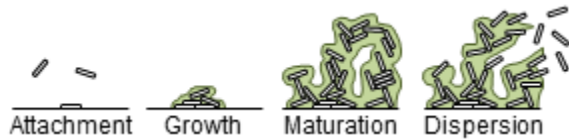
Figure 2. Simplified biofilm growth cycle. The rods represent the SOB, the green represents their metabolites and wastes. Note how the cells are embedded in the biofilm and how this growth form can increase surface area.
