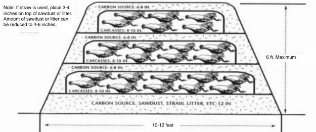
Figure 2. Cross-section of carcass composting in a windrow.
