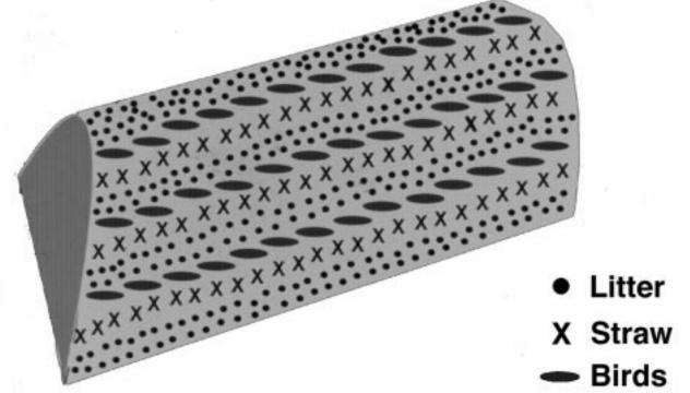
Figure 3. Completed catastrophic poultry composting windrow.
