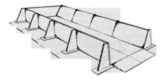
Figure 2. Stockplies With Permanent Ground Liners
