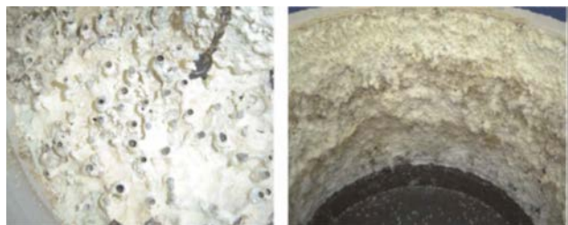
Figure 17. Accumulation of elemental sulfur on the walls and headspace of digester (Díaz, 2012)
