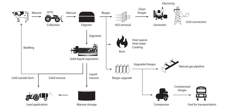
**Figure 3.** Scheme of the anaerobic digestion process and its potential products. Solid lines represent most common practices. Dotted lines represent alternative options for biogas and digestate processing and use.
