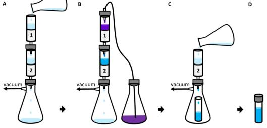
Figure 1. Schematic of sample purification/clean-up using SPE.
