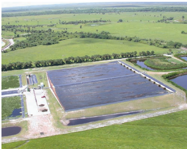
Figure 4. Aerial view of S-154 algal turf scrubber in central Florida. Photograph: Courtesy of HydroMentia, Inc.
